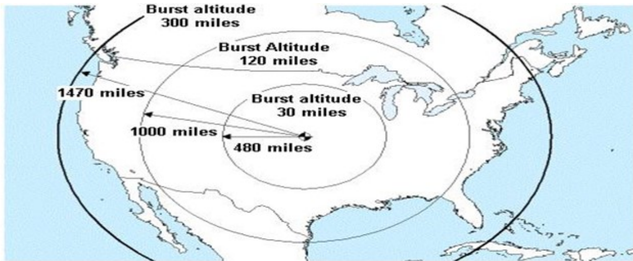
EMP AREA BY BURSTS AT 30, 120 and 300 MILES Gary Smith, "Electromagnetic Pulse Threats", testimony to House National Security Committee on July 16, 1997
